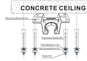
Note: According to the ceiling of different materials, use different screws to fix the hanging bracket. Don't fix the hanging bracket on the wood ceiling less than 12MM to prevent danger caused by
