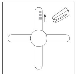
Place the clip on the blade that needs the counterweight and try the best place to place it, from the center to the tip of the blade, until the wobble disappears.
